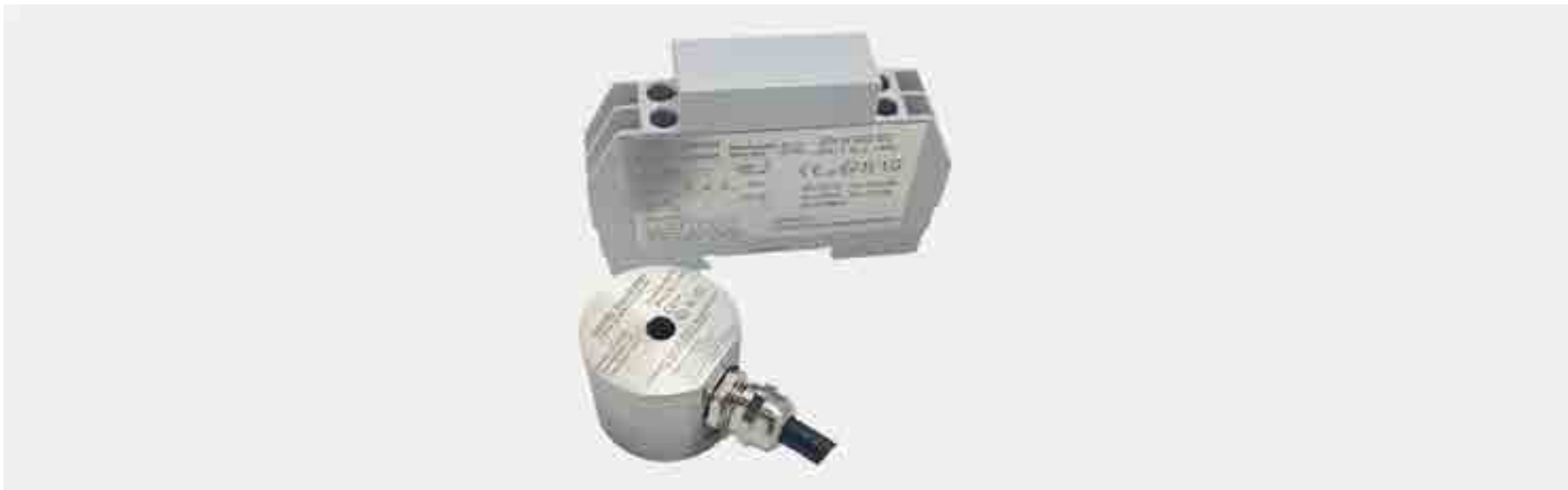
Model : LT-AV-EX · 4 ~ 20mA output LT-AV series is compatible with most PLC, DCS, SCADA and Plant Information (PI) systems. · It is designed to monitor overall vibration levels of auxiliary rotating machinery such as · This sensor must be used with certified safety barrier (IECEX/ATEX/KGS) : LT-AV-BARRIER
