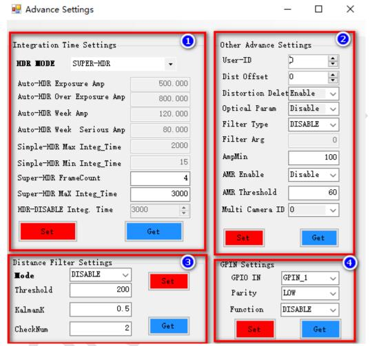
(1) Integration time mode setting: set the corresponding parameters according to the selected mode:
