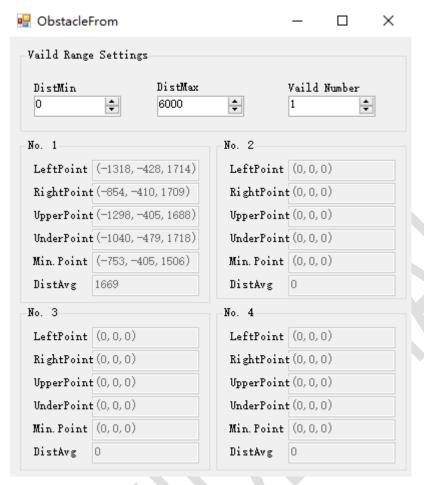
The extracted obstacle information is filtered by the minimum and maximum distance values, and the coordinate information of the obstacle feature pixel points is displayed according to the effective number, to facilitate the analysis of obstacles from near and far.
