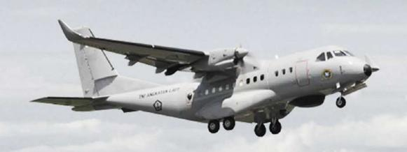
The CN235-220 multi-mission platform has proven to be a success in forward base operations on unpaved runway conditions.
