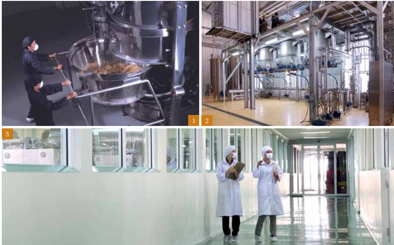
Production spaces in Sido Muncul's factory: 1) fluid bed dryer machine; 2) Percolator machine used for extraction; 3) Tolak Angin factory facilities.
