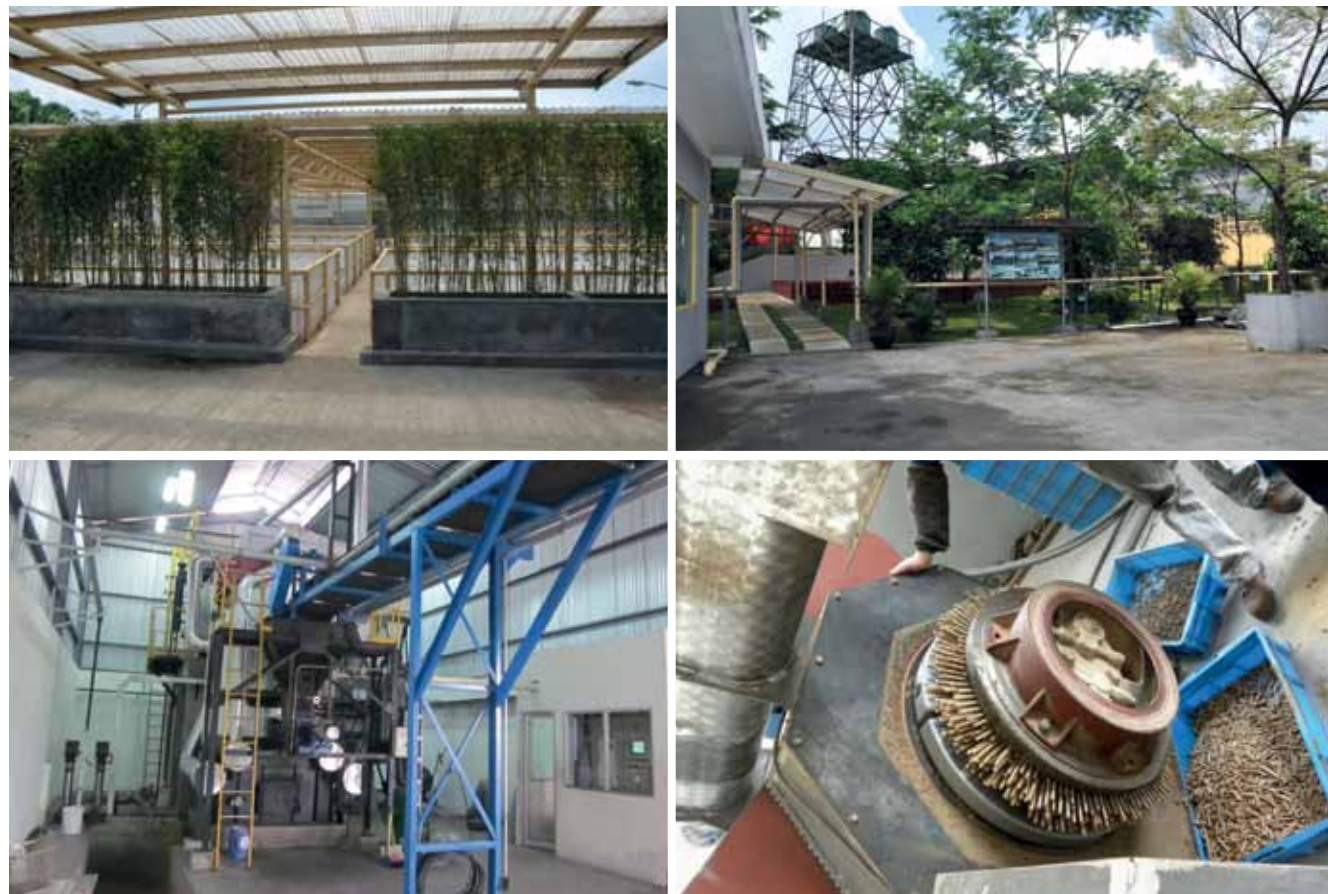
Bottom left: A dreg-processing machine. Bottom right: a pellet machine to turn dregs into solid pieces.
