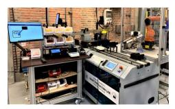
**Capture (2):** Proof of concept: Research team has connected a KUKA robot to a Microsoft Azure cloud of the LEGO Group via an edge interface of the Munich-based IoT specialist Device Insight.
