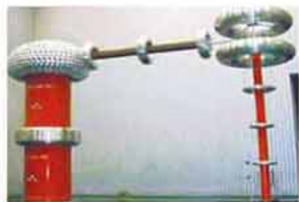
600kV Power Frequency Test Transformer
