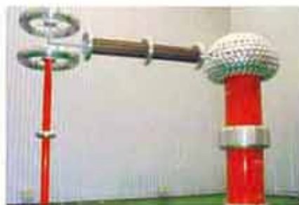
1000kV Power Frequency Test Transformer
