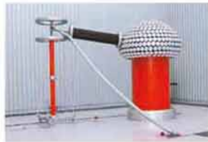
300kV Power Frequency Test Transformer
