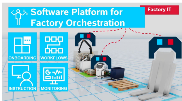
Bild 4: The asset administration shell functions as a standardized digital twin for all automation components and solutions - both from Bosch Rexroth and from other manufacturers. Users orchestrate their brownfield and greenfield equipment graphically in ISO/IEC standardized process models, independent of lot size, with the new individually adaptable software platform for flexible and changeable manufacturing, and without downtimes. (Bildquelle: Bosch Rexroth AG)
