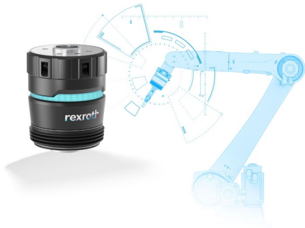
Image 2: Sensor-based compensation unit for articulated and linear robots: The Smart Flex Effector increases precision and productivity, avoids errors and allows greater automation. (Image source: Bosch Rexroth AG)
