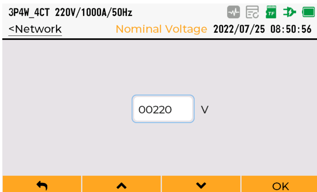
Figure 5-7 Nominal voltage configuration
