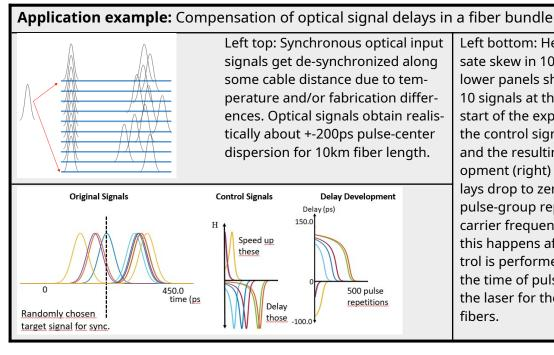
Left bottom: Here we compensate skew in 10 fibers. The lower panels show the original 10 signals at the receiver at start of the experiment (left), the control signals (middle) and the resulting delay development (right) where all delays drop to zero at about 500 pulse-group repetitions. At a carrier frequency of 10GHz this happens after 50ns. Control is performed by adjusting the time of pulse insertion by the laser for the different fibers.
