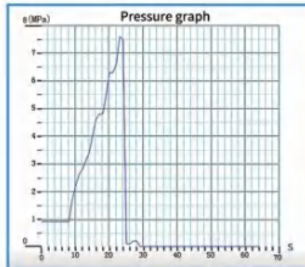
Single sphere rubber expansion joint burst testing
