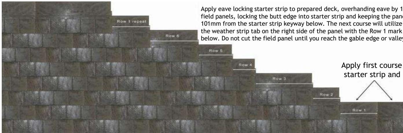
Measurements are taken from the outside edge of weather strip tab on the right side of the panel
