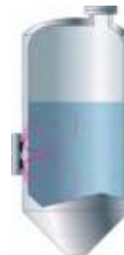
Figure 2.48: Quantum Sensing for detection medium through the steel wall (Source: Endress+Hauser SE+Co. KG)
