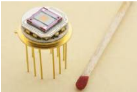
Figure 2.61: Pyroelectric detector module with tunable FP filter mounted on top of the detector (Source: InfraTec, www.infratec.de )
