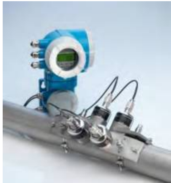
Figure 2.52: Ultrasonic clamp-on flowmeter with two sound paths, providing good accuracy and easy installation, especially in difficult installations with limited space
