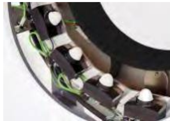
Figure 2.68: High-accuracy radar sensors arranged in a circle for measuring the wall thickness of pipes (Source: INOEX GmbH)
