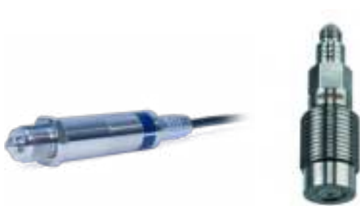
Figure 2.11: Left: High Pressure sensor foil type strain gauge: Pressure Sensor P3 Top Class BlueLine (Source: HBK); right: piezoelectric high pressure sensor 6213B for dynamic measurements up to 10 kbar (Source © 2024 Kistler Group)
