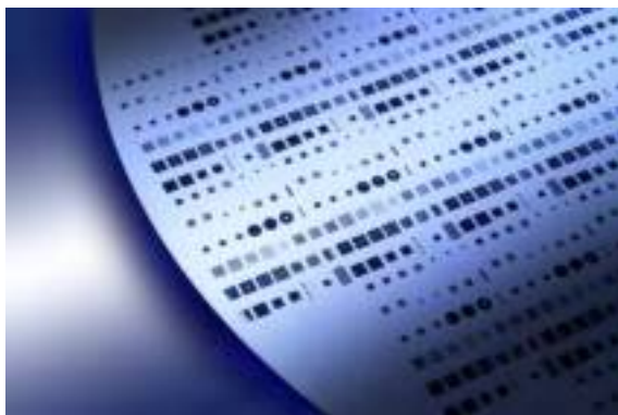
Figure 5.15: 200 mm silicon wafer with integrated NdFeB magnets. The magnets have lateral dimensions between 40 \mu\text{m} and 2 mm and are 500 \mu\text{m} thick. (Source: Bodo Schmidt)
