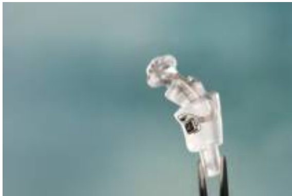
Figure 5.1 Pressure sensor with aerosol jet printed wiring on additively manufactured substrate (Source: Hahn-Schickard/Bernd Müller)
