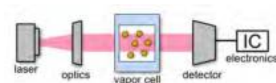
Figure 5.18: Schematic principle of an alkali vapor cell
