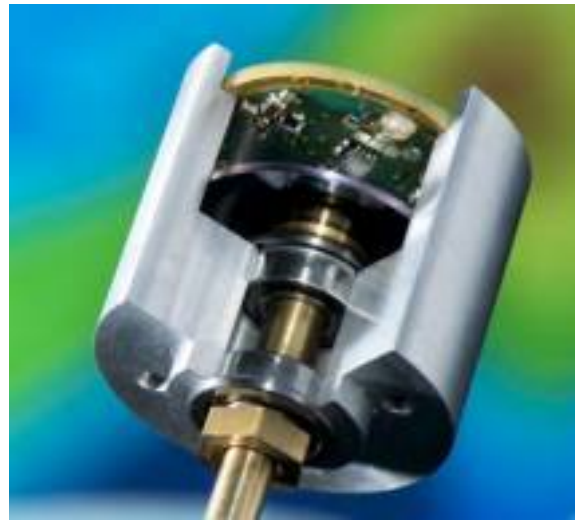
Figure 5.9 Optical encoder with micro-structured polymer components (Source: Hahn-Schickard/Bernd Müller)
