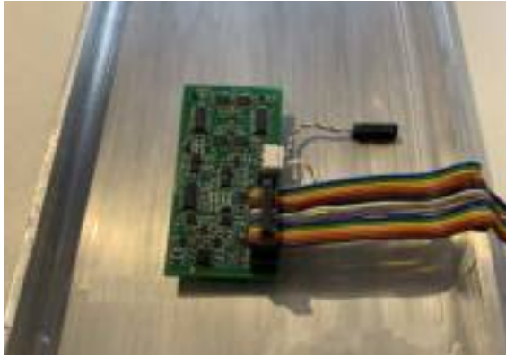
Figure 2.32: Structural current sensor with both Hall and inductive current sensing on an aircraft structural beam [Blagojevic et al., 2023] (Source: SENIS AG).
