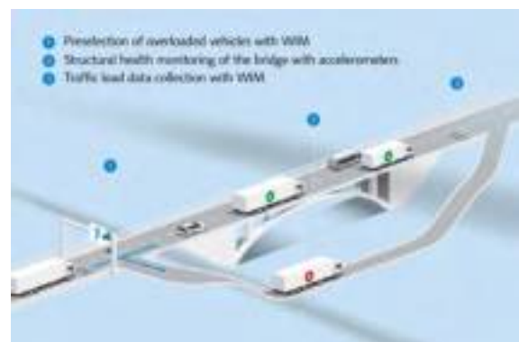
Figure 4.16 Vehicle-load monitoring for bridge protection. The load is measured with a so-called weight-in-motion sensor (WIM), which is based on piezoelectric technology (Source: © 2024 Kistler Group)
