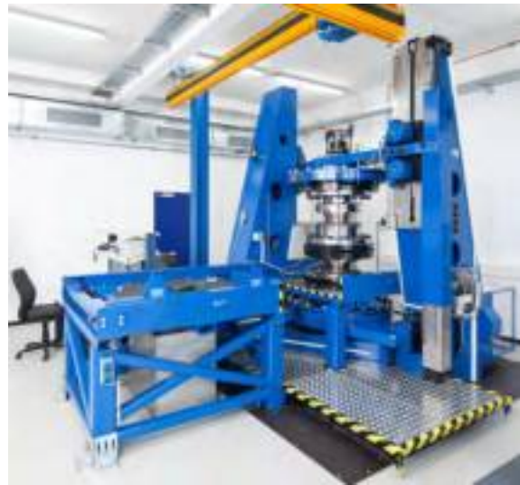
Figure 2.20: 400 kN·m Torque calibration device, (Source: HBK)
