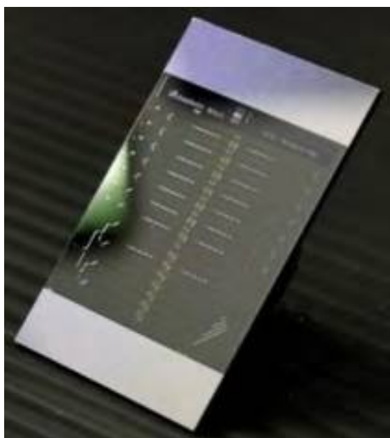
Figure 3.12: Silicon chip-integrated photonics as biosensors for optical detection of biomolecules (Source; Dr. Florenta Costache, Fraunhofer IPMS)
