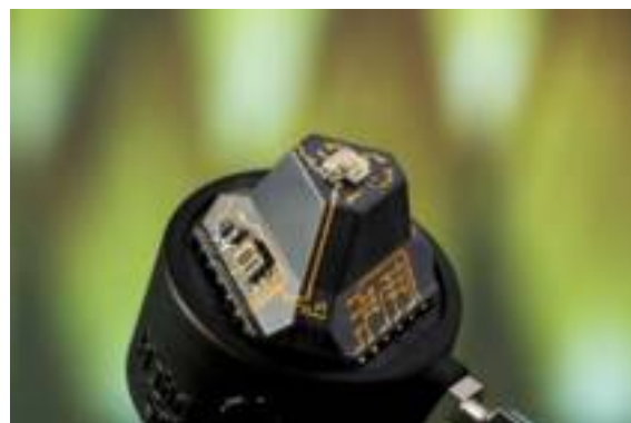
Figure 5.4 Three-dimensional circuit carrier with spatially oriented light sensors (Source: Hahn-Schickard/Bernd Müller)
