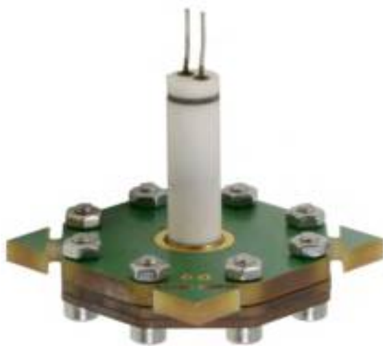
Figure 3.3 Non-radioactive X-ECD based on a high energy photon source not bound to any regulatory restrictions and manufactured at low cost from printed circuit boards with detection limits in the lower ppt range and a linear range of up to four orders of magnitude. (Source: Maximilian Küddelsmann)
