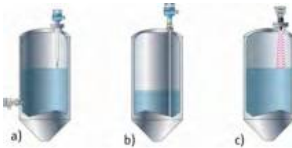
Figure 2.45: Level principles, a) point level; b) contact continuous; c) non-contact continuous (Source: Endress+Hauser SE+Co. KG)
