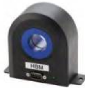
Figure 2.31: Fluxgate current transducer Hottinger Brüel Kjaer CTS200ID, manufactured by DaniSense, (Source: HBK)
