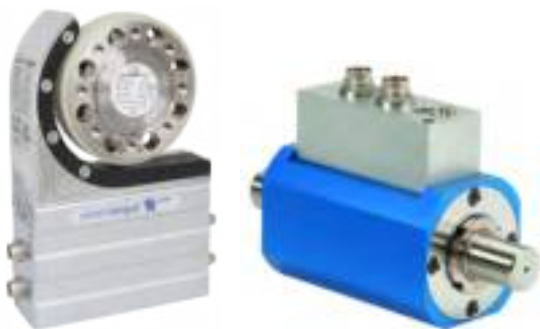
Figure 2.17: left: Flange type torque transducer T12HP (Source: HBK); right: Shaft type sensor 4503B, for high-speed torque measurements, both based on foil type strain gauges (Source © 2024 Kistler Group)
