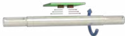
Figure 2.18: Non-contact torque measurement (Source: NCTE AG)
