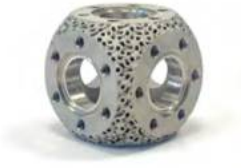
Figure 5.26: Additively manufactured vacuum chamber for cold-atom experiments with a gyroid lattice for weight reduction (Source: IMPT)
