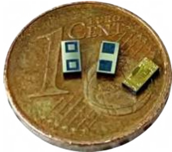
Figure 5.16: 3D Hall sensor with NdFeB magnets integrated into the substrate at wafer level on the back (Source: Florian Ziegler)
