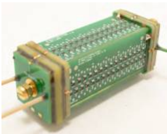
Figure 3.2 Low-cost, high-performance DTIMS made from printed circuit boards with high resolving power of R = 60 and detection limits in the low ppt range within one second of measuring time but short drift length of just 40 mm. (Source: Alexander Bohnhorst)
