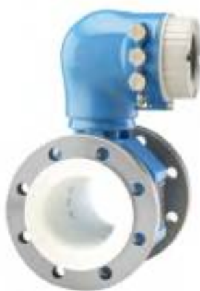
Figure 2.51: Magnetic inductive flowmeter; three pairs of electrodes allow for installation independent of flow disturbances, like bends or valves.
