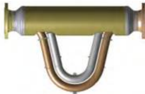
Figure 2.55: Inside view of the 4-tube meter (see Figure 2.54); 2 different oscillation frequencies allow for additional information and diagnostics, as well as compensation of errors due to aeration of the measured product
