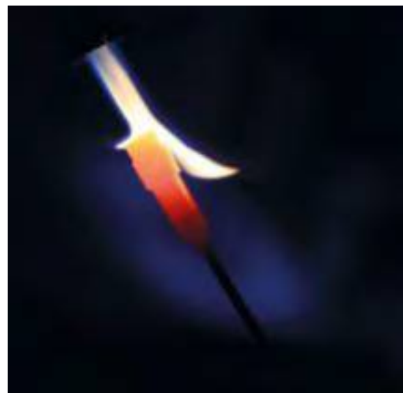
Figure 5.22. Sensor providing reliable measurement data under extreme conditions (red glowing metal casing). Temperatures of 700\text{ }^{\circ}\text{C} for long-lasting pressure and acceleration measurements are highly demanding requirements for a suitable sensor design. In some cases, even higher temperatures for short-term measurements are possible. (Source © Kistler Group 2024)
