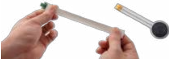
Figure 6.3 FlexSense – Electroactive Polymer (EAP) stretch and pressure sensors (Source: Alexander York, matelligent IDEAS)
